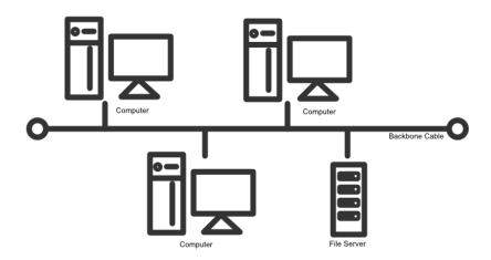
In a bus topology, all the terminals (devices) are connected to a backbone cable, the ends of which are plugged into a terminator.
